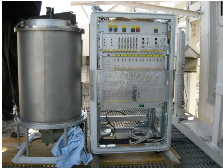
Figure 2.3: The cryogenic part (left) and the non cryogenic part (right) of the receiver.
