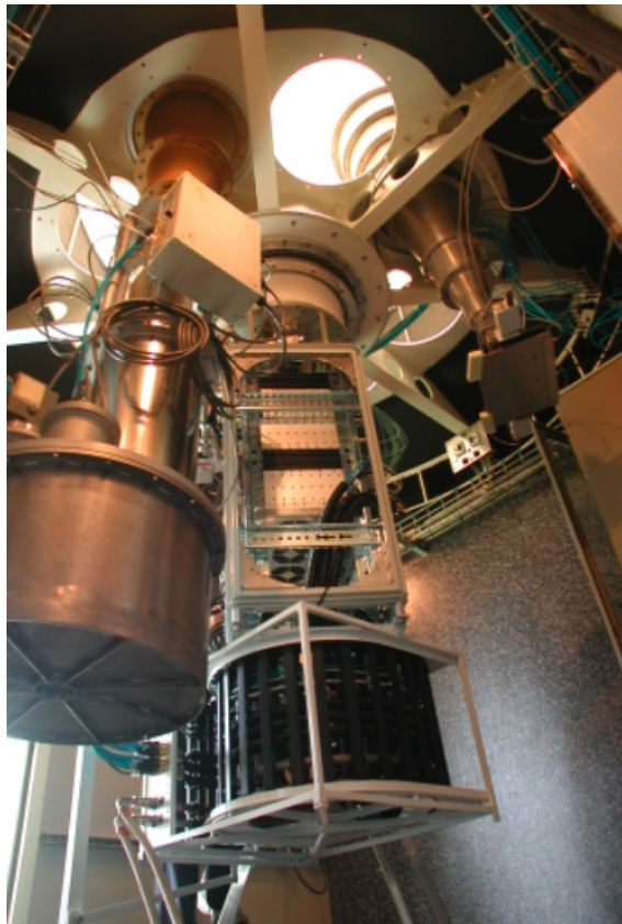
Figure 2.4: Final installation of the MF receiver at the cassegrain focus of Medicina 32-m dish.
