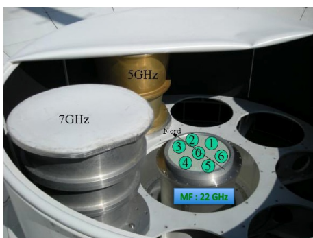
(a) Top view of MF receiver (feeds numbered) installed in the central bay of the cassegrain focus of Medicina 32-m dish.
