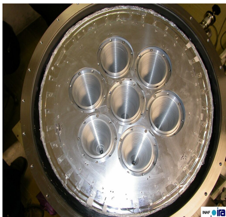
(a) A photograph of the K-band multi-feed receiver (cluster of horns) designed for the new Sardinia Radio Telescope. The receiver spans a frequency range of 18-26.5 GHz. Photograph courtesy, Istituto di Radioastronomia-INAF, Italy.
