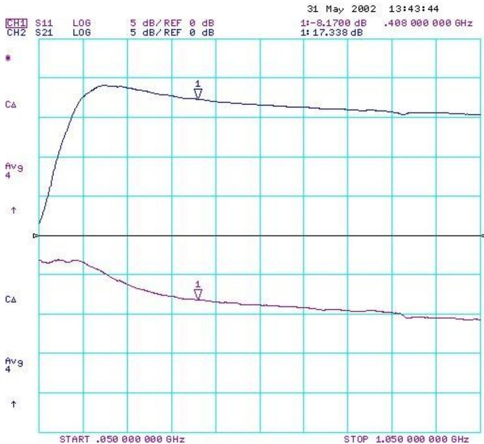
**Figure 6.12: Measured S11 and S21 of the second stage prototype**
