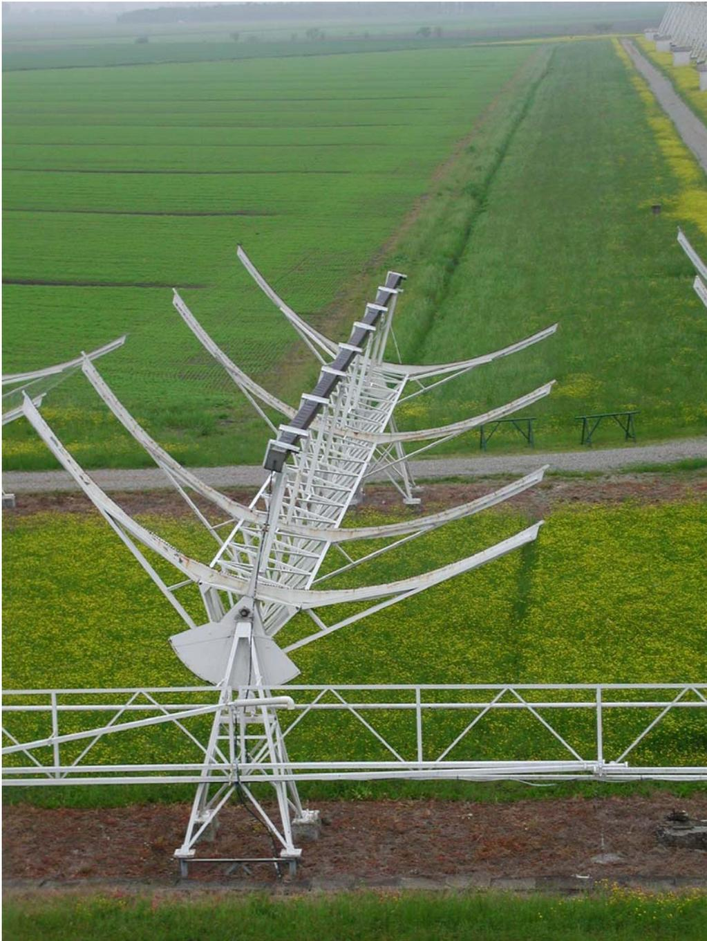
Fig.2.2.1: A single N/S cylindric element used for BEST-1
