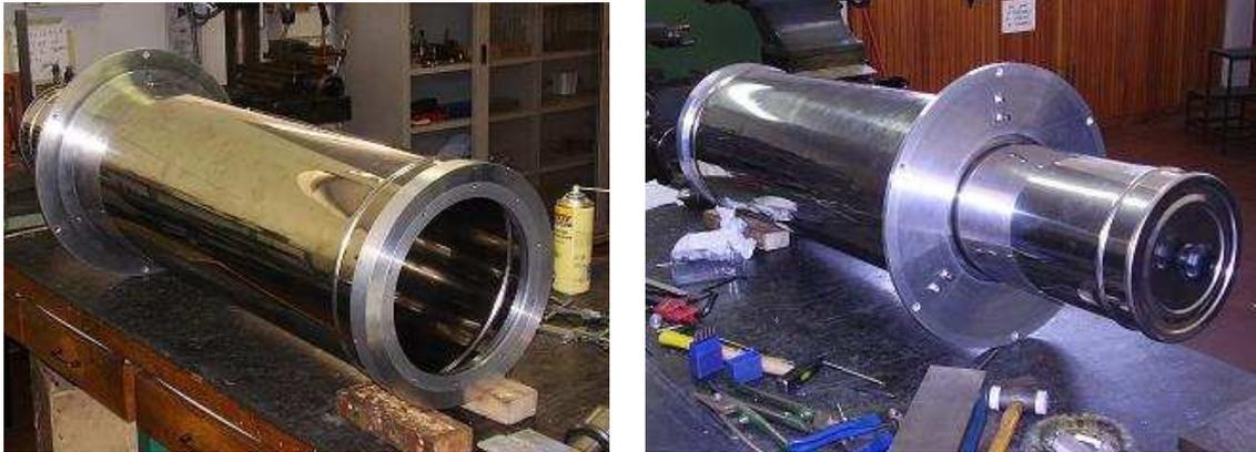
**Fig. 3: The top (left) and bottom (right) stainless steel telescope covers with the TA/RT interface.**
