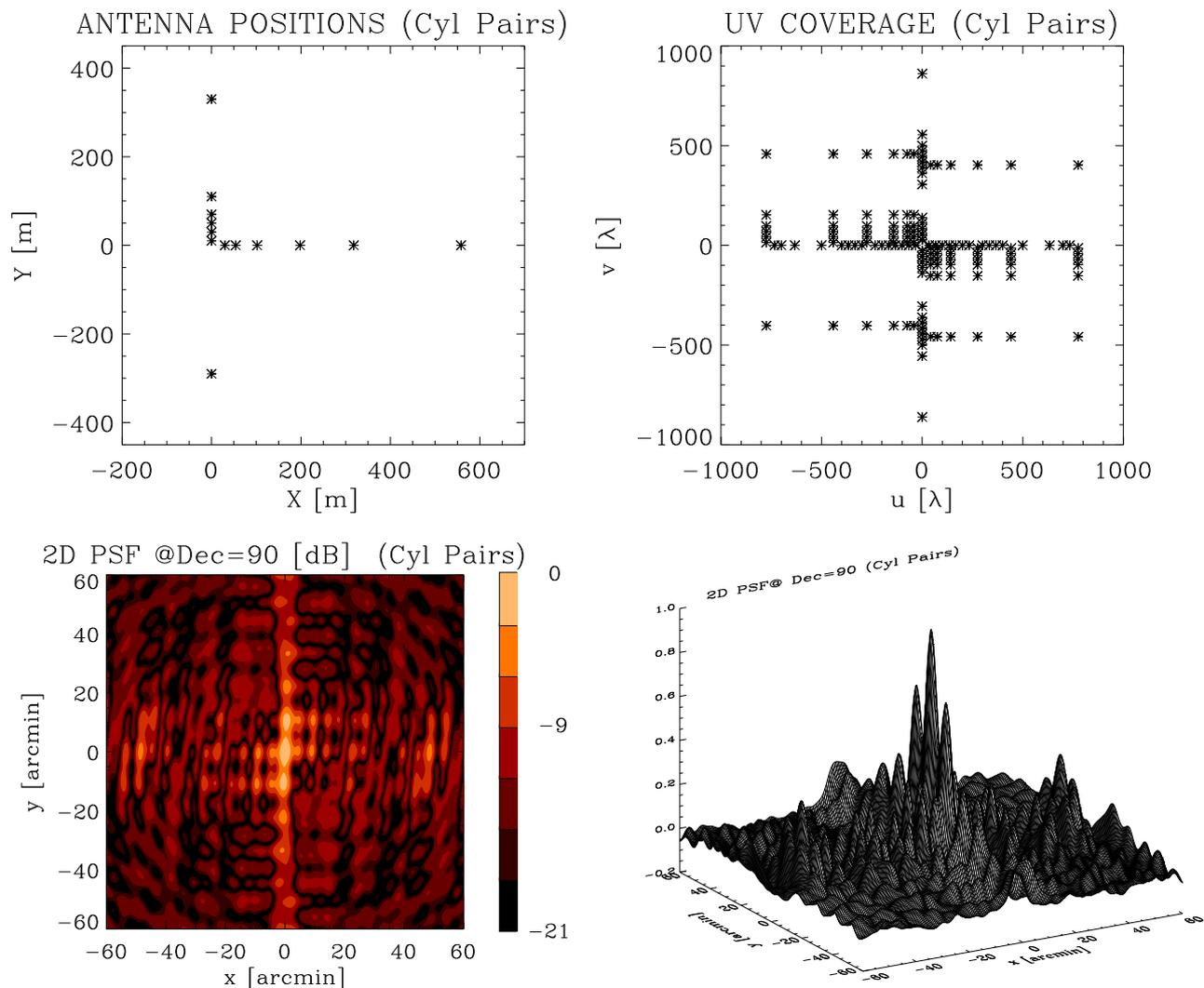
Figure 6: **Top:** Antenna positions (right) and uv-plane coverage (right) for the cylinder pairs case (other details are as for Fig. 4). **Bottom:** As for Fig. 5 except that it is for the cylinder pairs configuration and for the Dec=90° only. The main secondary lobes of the NS direction are high, being at about -2dB.
