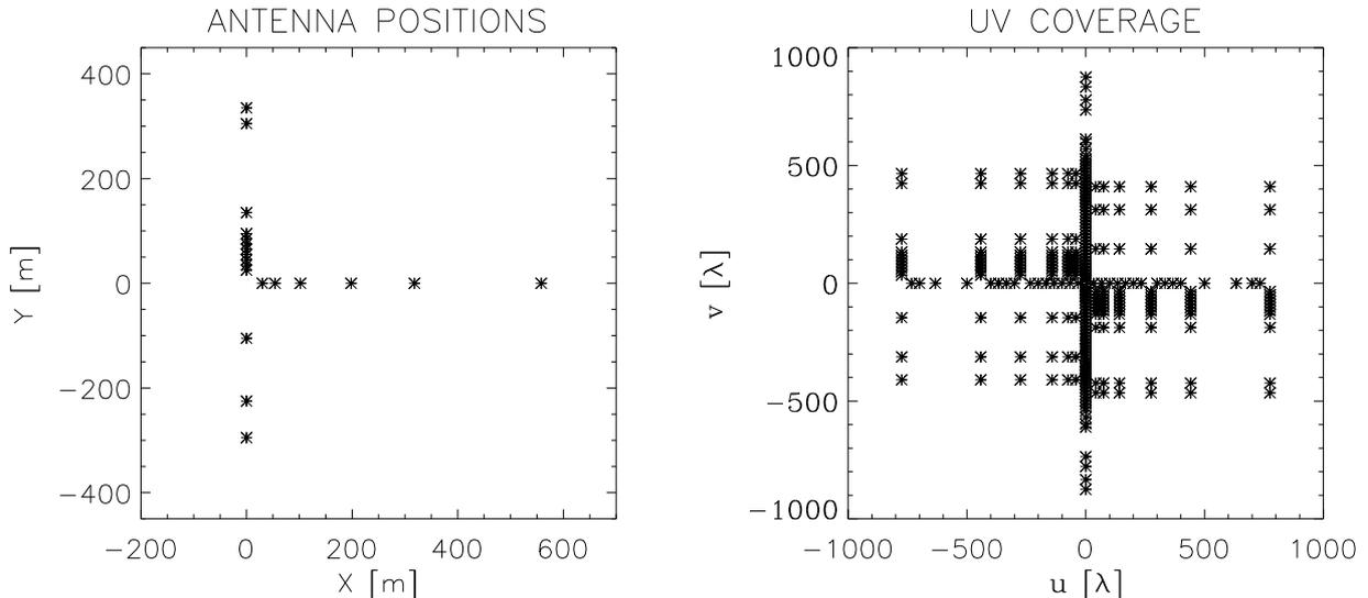
Figure 4: Antenna positions (left) and uv-plane coverage (right) of the configuration which optimizes the Northern Cross beam response. The uv-plane coverage is given in case of instantaneous observation of a source at transit (Hour Angle = 0) and at the Zenith (unit is wavelength:  $\lambda = 0.735$  m)
