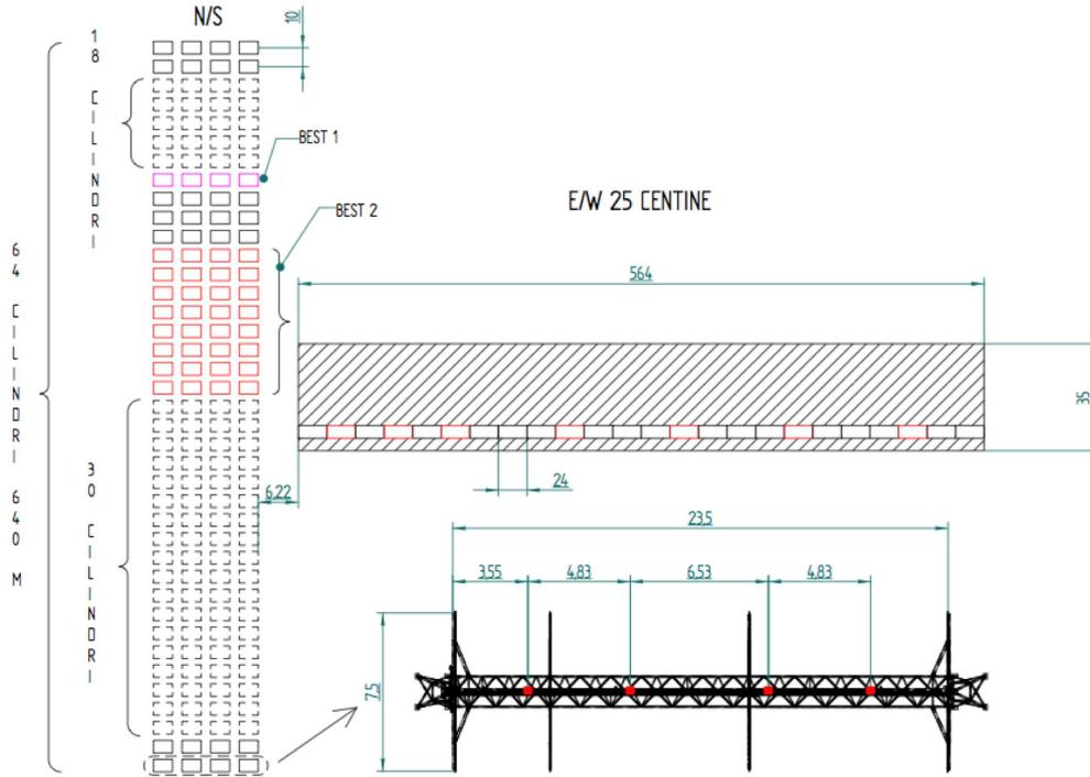
Figure 1: NS Cylinders and EW arm of the Northern Cross radiotelescope. The cylinders used for BEST-1 and BEST-2 phases are also reported.
