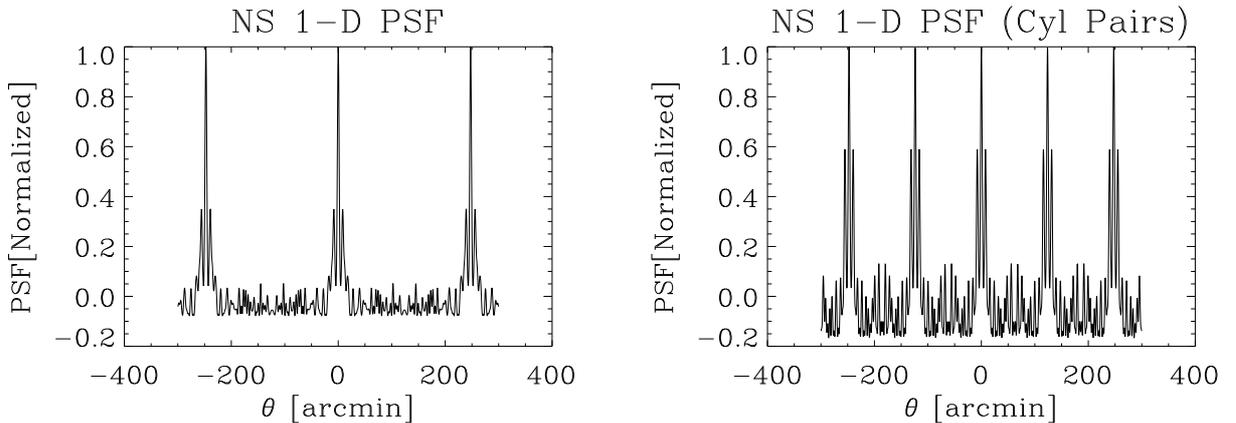
Figure 3: **Left:** 1-D PSF of the NS arm of the best configuration: this has been found out by assuming to be free to chose any of the available cylinders for the 5 new antennas to be added to BEST-1 and BEST-2 (see text). **Right:** as for the Left panel, except assuming the NS cylinder to be paired 2-by-2. This does not leave almost any freedom to locate the new 5 cylinders: one has to be paired to BEST-1, and the other four are to realize two pairs, one at each end of the NS arm (see text).
