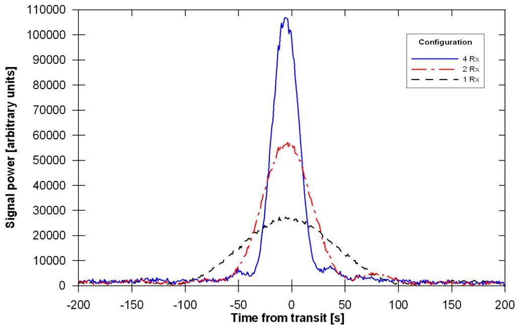
Fig. 41: Transit of Taurus-A observed by a single E-W receiver (dashed black line), by a synthesized beam of 2 receivers (dashed dotted red line) and of 4 receivers (continuous blue line)
