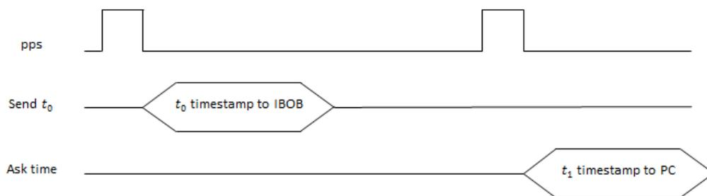
Fig. 19: Time diagram of the time update procedure
