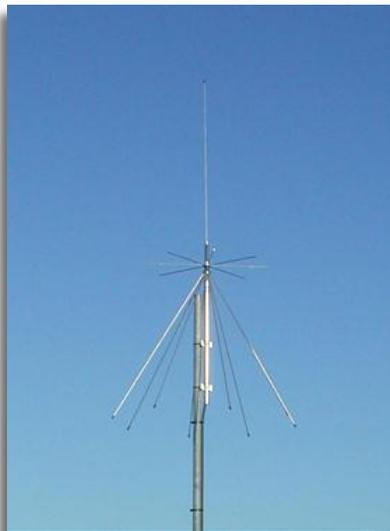
Fig. 30: Omnidirectional Antenna
