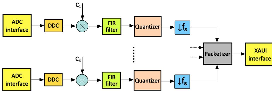
Fig. 15: IBOB firmware architecture
