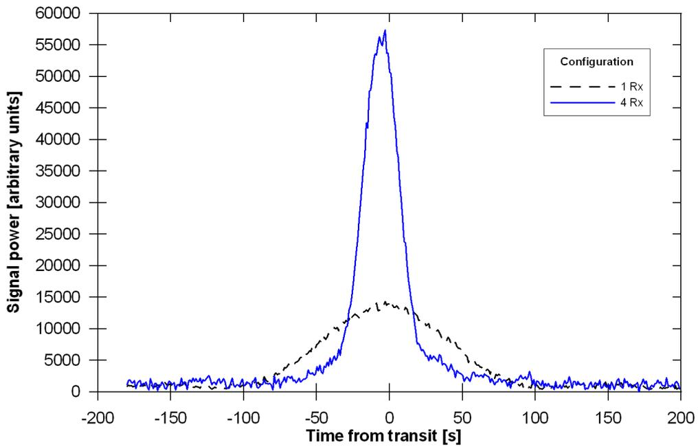
Fig. 40: Transit of Virgo-A observed by a single E-W receiver (dashed black line) and by a synthesized beam of 4 receivers (continuous blue line).
