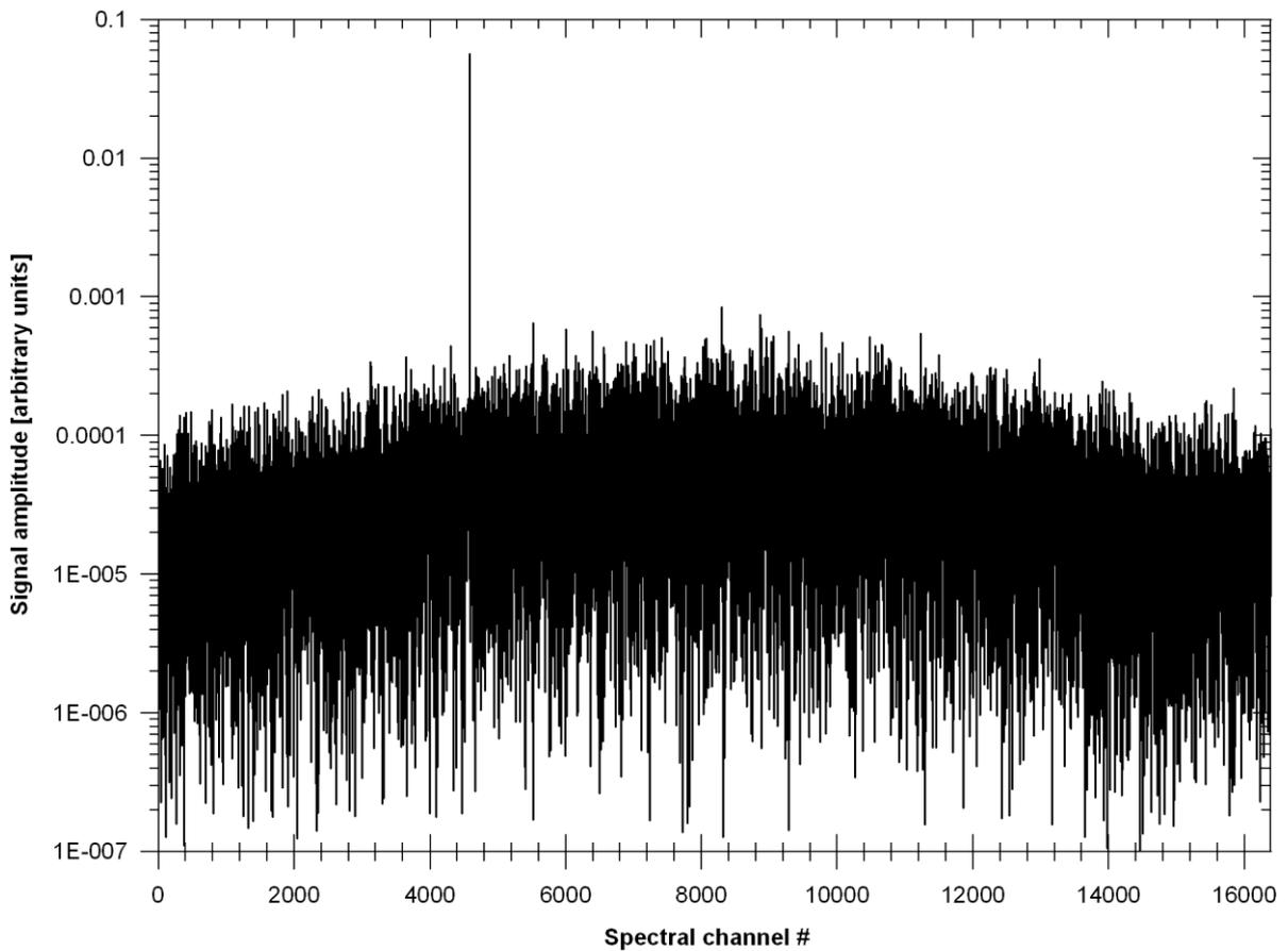
*Fig. 42: Spectrum of the echo from the target NEXTSAT detected during on 2012 December 17 at 09:01:06.25 UT. The spectral window is centred at the transmitting frequency. Due to the extremely high SNR of the echo, the signal amplitude is plotted in logarithmic scale.*
