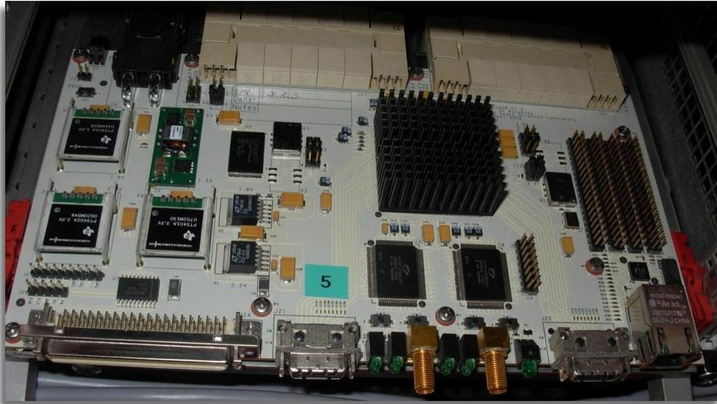
Fig. 3: The IBOB board, you can see on the top the 2 ZDOKs for A/D boards, two CX4 connectors below, JTAG pins on the left, while the Xilinx Virtex 2 Pro is behind the cooler
