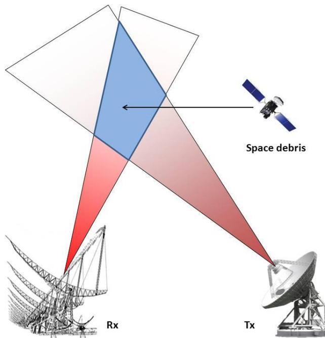
Fig. 1: Bistatic radar configuration geometry.
