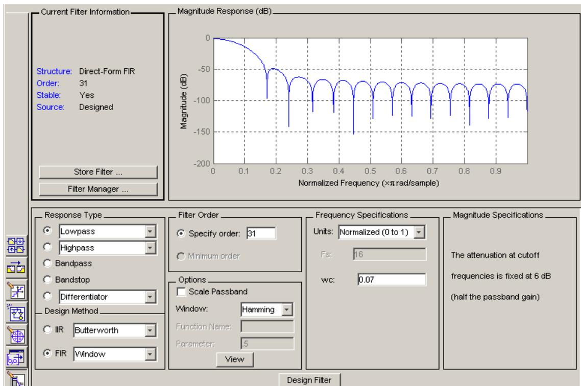
Fig. 18: Design parameters of the FIR filter synthesized in the IBOB.
