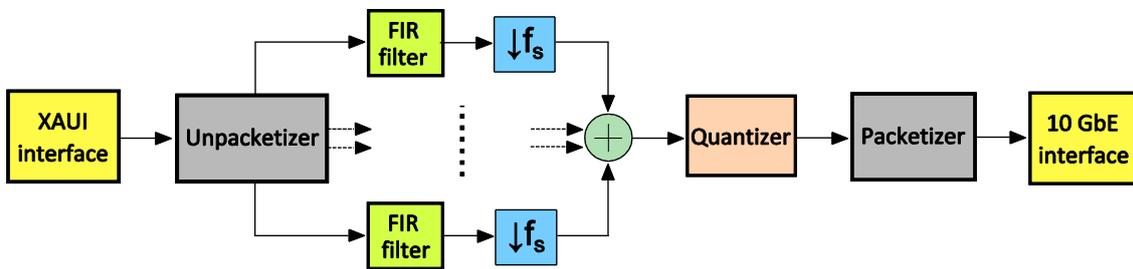
Fig. 24: BEE2 firmware architecture
