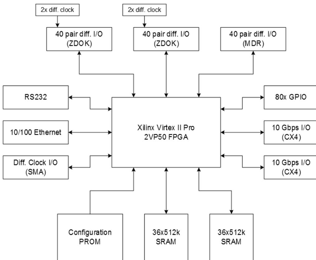
Fig. 2: Block diagram of the Ibob board general architecture
