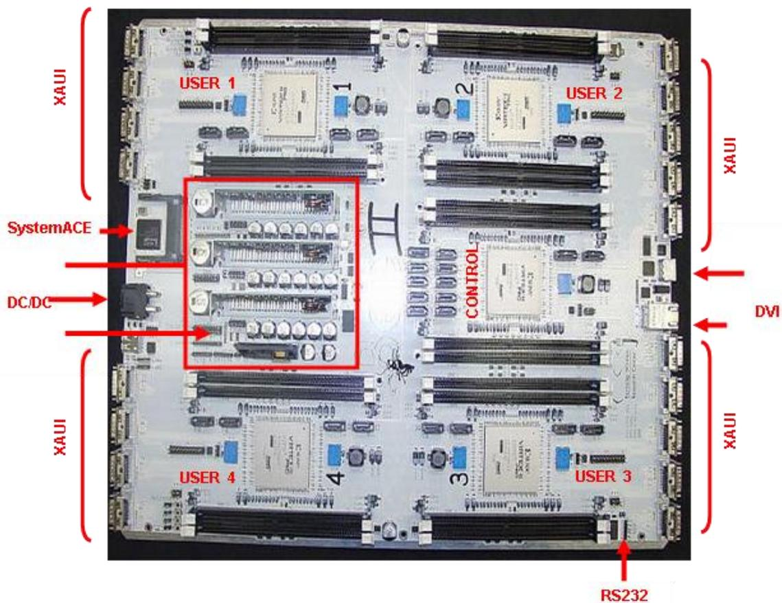
Fig. 5: A picture of the BEE2 board whose principal components are pointed out.
