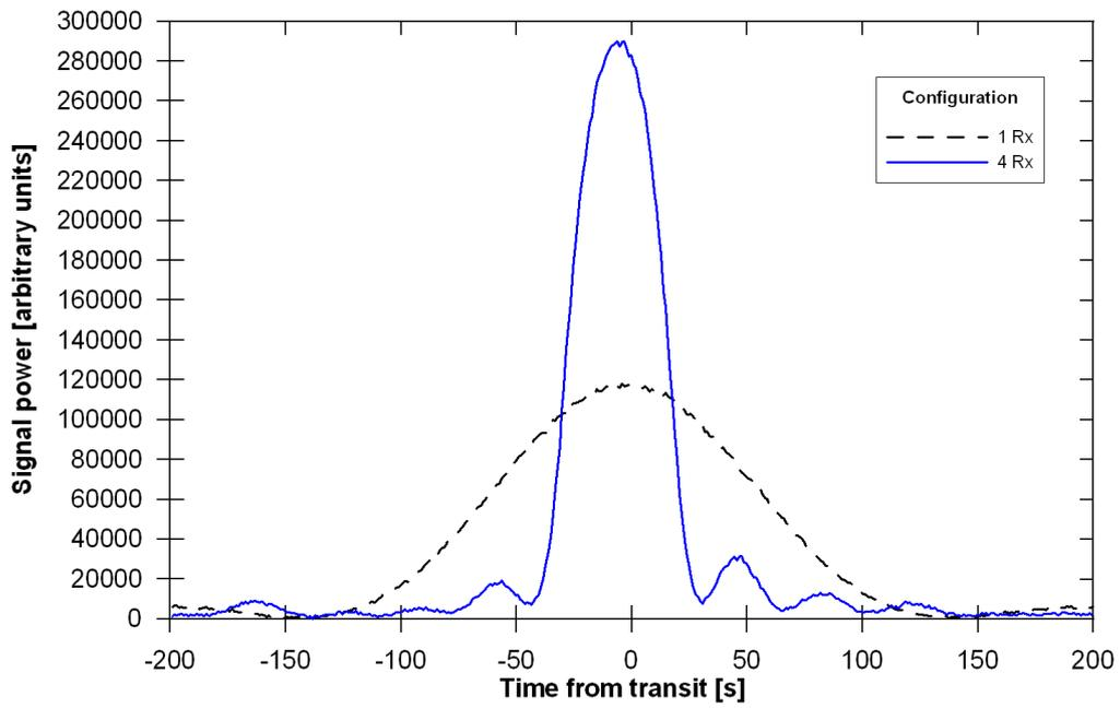
Fig. 39: Transit of Cygnus-A observed by a single E-W receiver (dashed black line) and by a synthesized beam of 4 receivers (continuous blue line).
