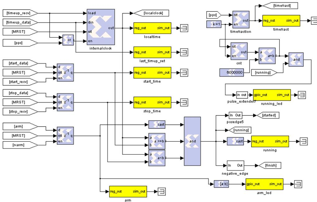
Fig. 20: IBOB Timing registers
