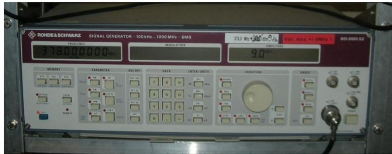
Fig. 12: Picture of the Local Oscillator set to 378MHz in input to the MIXER to generate a IF of 30MHz
