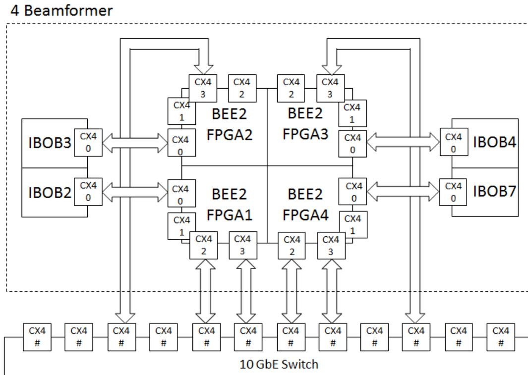
Fig. 11: 4 Parallel Beamformer System Connection Scheme
