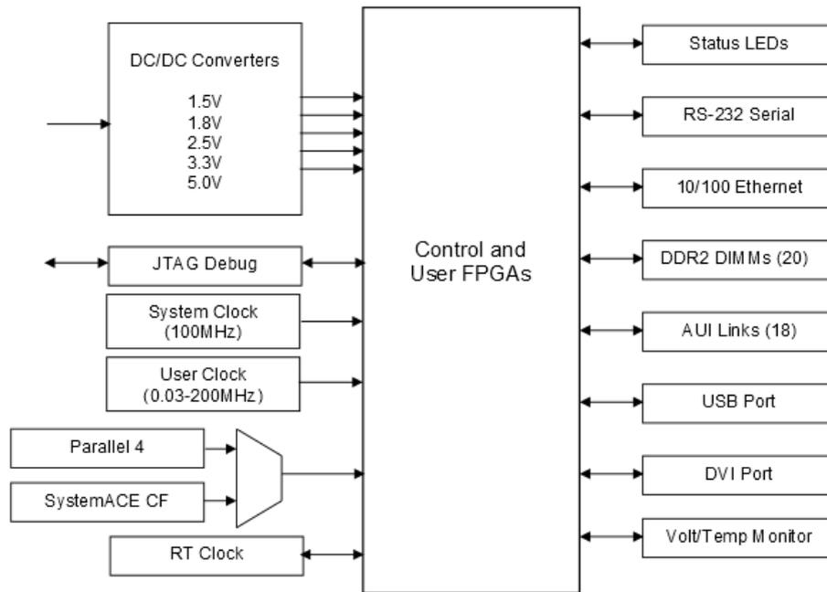
Fig. 6: Block diagram of the BEE2 board general architecture
