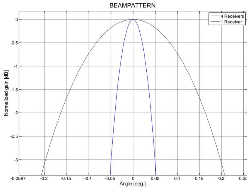
Fig. 38: Normalized E-plane power patterns calculated for a single E-W receiver (dotted black line) and for a synthesized beam of 4 receivers (continuous blue line).
