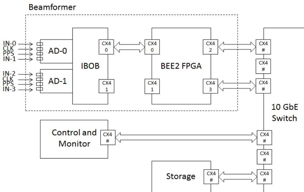
Fig. 10: Basic connection scheme
