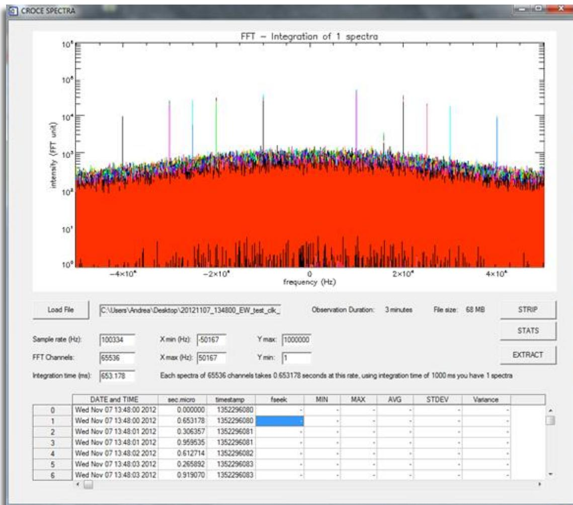
Fig. 34: Overplotting FFTs of the entire file you can recognize the frequencies used for the test.
