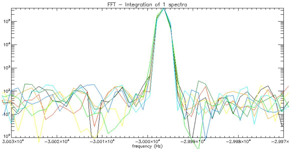
Fig. 35: Frequency 407.970kHz sampled using the HP 8657B as clock sampler.
