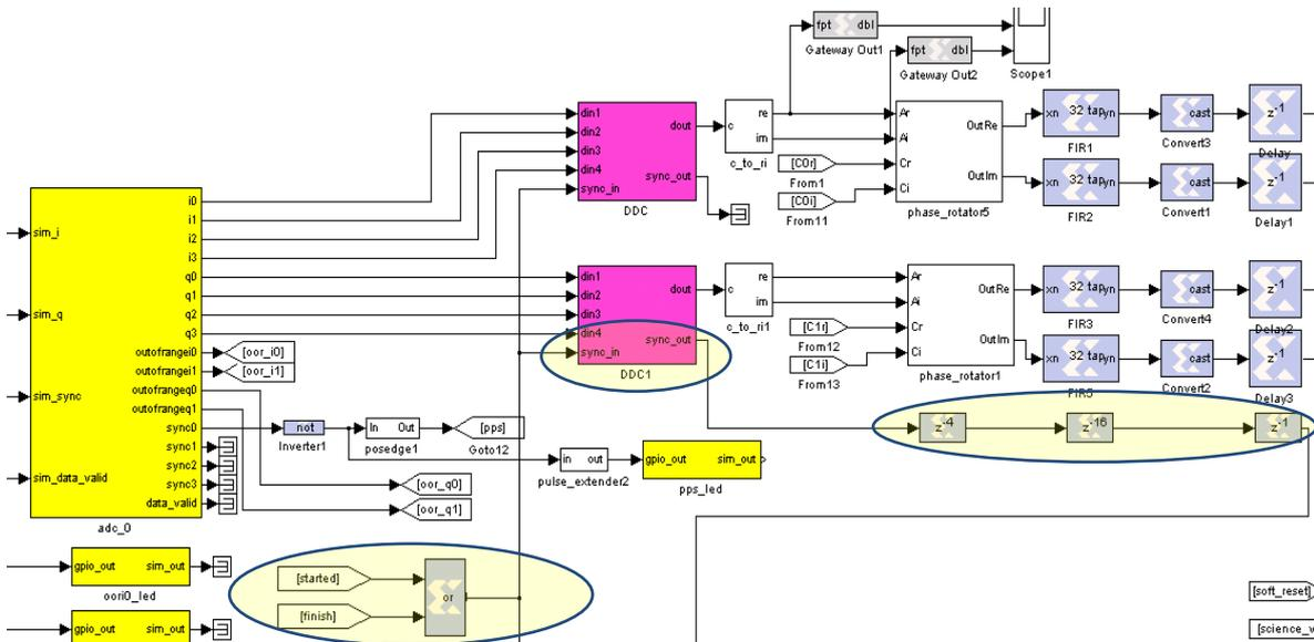
Fig. 21: Propagating the sync signal with intermediate block latencies
