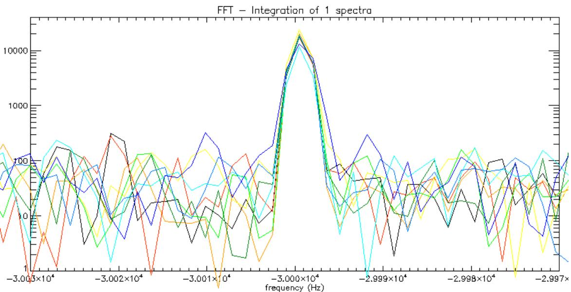
Fig. 36: Frequency 407.970kHz sampled using the Rohde&Schwarz SMX as clock sampler.
