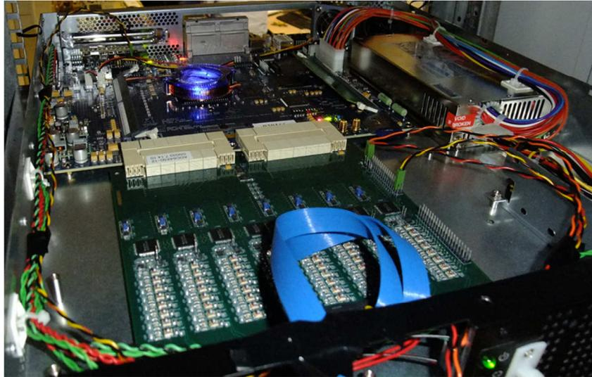
**Fig. 8 - The ROACH board, a XILINX Virtex-5 SX95T FPGA board, with the 64 input ADC connected via two Z-DOK connectors.**
