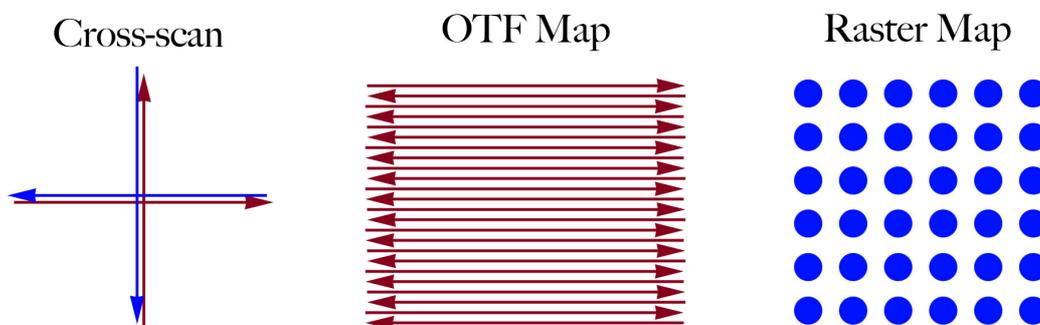
In the case of cross-scan, a subscan is a single arrow (a line across the target), four arrows – i.e. two full crosses – constitute the schema which might be repeated as many times as needed within the scan.
