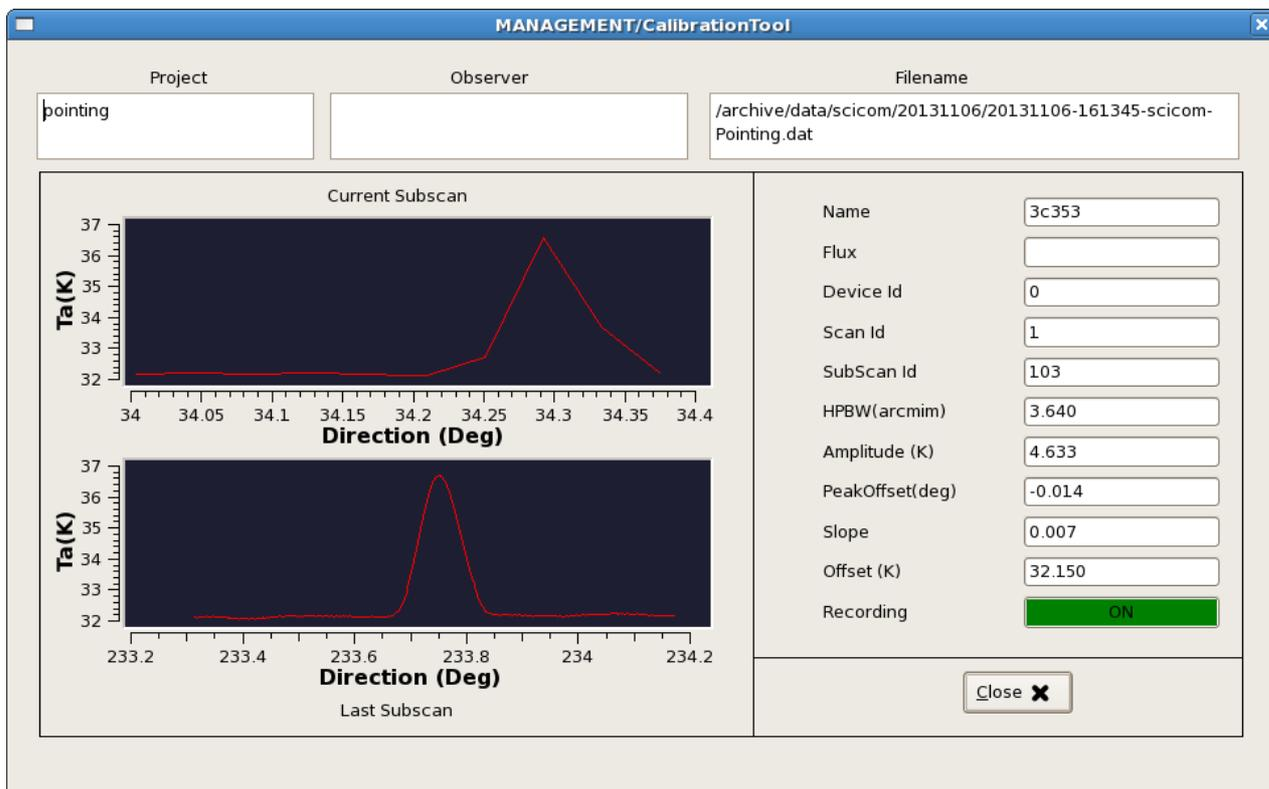
Notice that, in this client, the subscan currently being acquired is shown *in real-time* (upper plot), even if in a low-res version. Under this display, the last completed subscan, in its full sampling, is shown.
