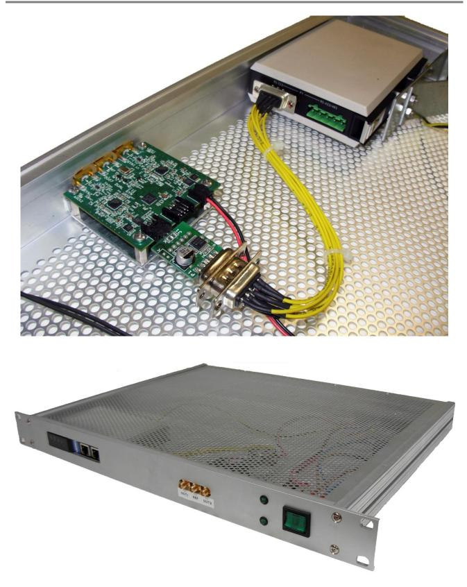
The front panel provides a button switch to power on and off the module, two green LEDs indicating if 5 Volts modules are powered, the SMA connectors for RF input/output of the clock synthesizer ant the Ethernet port of the TCP/RS-232 converter. On the rear panel you will find the 220V socket with the fuse.
