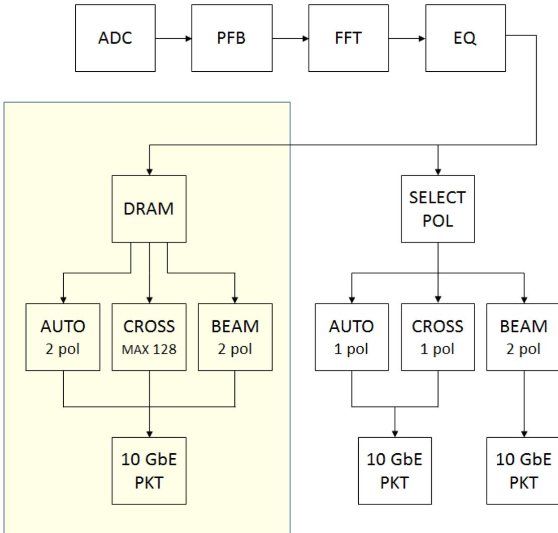
The first row of the block diagram is the common part between the two independent systems producing more or less the same output with different resolution (bit quantization). There are 4 parallel streams of antenna spectra (organized by antennas and not by frequency channels) where few logic blocks catch the 512<sup>th</sup> channel where we expect to find the sine wave transmitted by the drone at 408 MHz.
