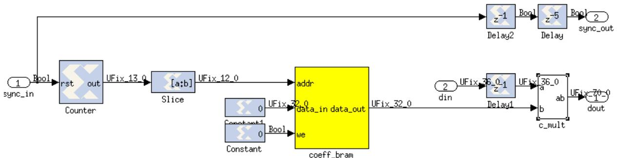
The phase correction factor is a complex number having the real and imaginary part written has a fixed point 16.15 each. The data output is a complex number where real and imaginary part have the format 35.32 each. This 70 bit number will be the final number which will be used for the auto correlation and cross correlation products in the new firmware, while the old branch of the firmware will keep a quantized data of 8.7 bit for real and imaginary part each.
