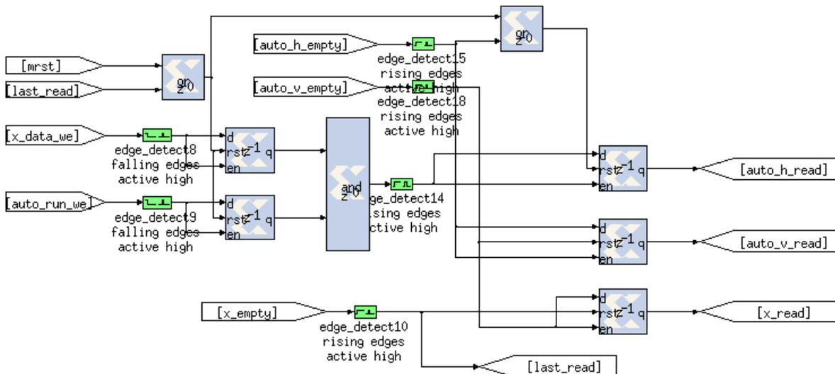
A big multiplexer is demanded to switch between data flow and the selection of the mux input is shown on the next pictures.
