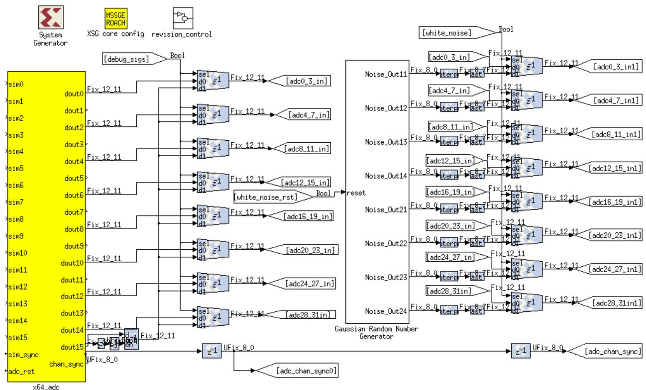
The ADC yellow block is a Simulink block written by the CASPER group that allows to address the ADC64in board. It produces 16 digital output in a clock cycle and the 64 parallel outputs in 4 clock cycles. Running the FPGA at least 4 times faster than the ADC board (which will have a dedicated synthesized clock signal) you will be able to manage up to 64 different input. The format of the data is Fix\_12\_11 which means a fixed point number of 12 bits with 11 bit of decimals.
