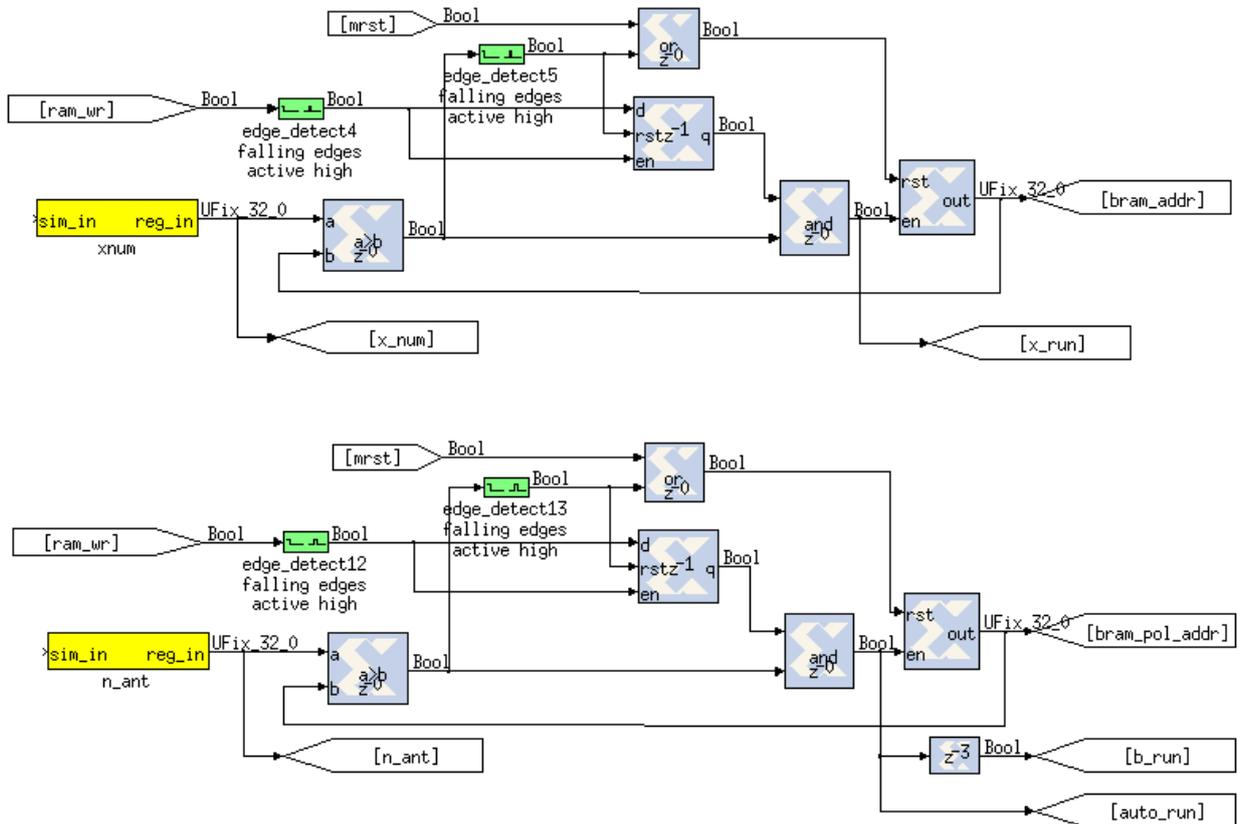
As seen in the above pictures, “bram\_pol\_addr” and “bram\_addr” values are the addresses for the BRAM, while BRAM output signals called “ram\_adrxxx” are the addresses for the dual port RAMs.
