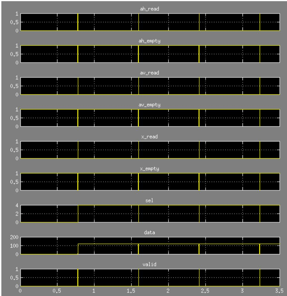
All engines have finished to compute their products and now the FIFOs are full of data and must be emptied. A few logic blocks produce, in sequence, the read enable signals to read the FIFO data in the order: AUTO-H, AUTO-V, CROSS. The next pictures shows how it is done.
