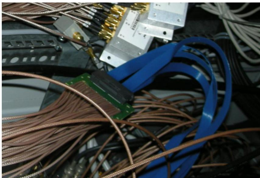
The next picture shows the cabling, the black coaxial cables are the input signals coming from the optical receivers (16 MHz of bandwidth centered at 30 MHz), the metallic boxes are some splitter used to close to 50 Ohm a set of unused ADC inputs.
