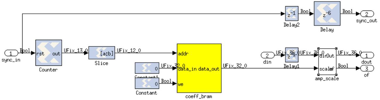
The previous picture show in details the amplitude equalization stage: going into the Simulink subsystem you will find the BRAM yellow block, and another subsystem “amp\_scale” making the multiplication.
