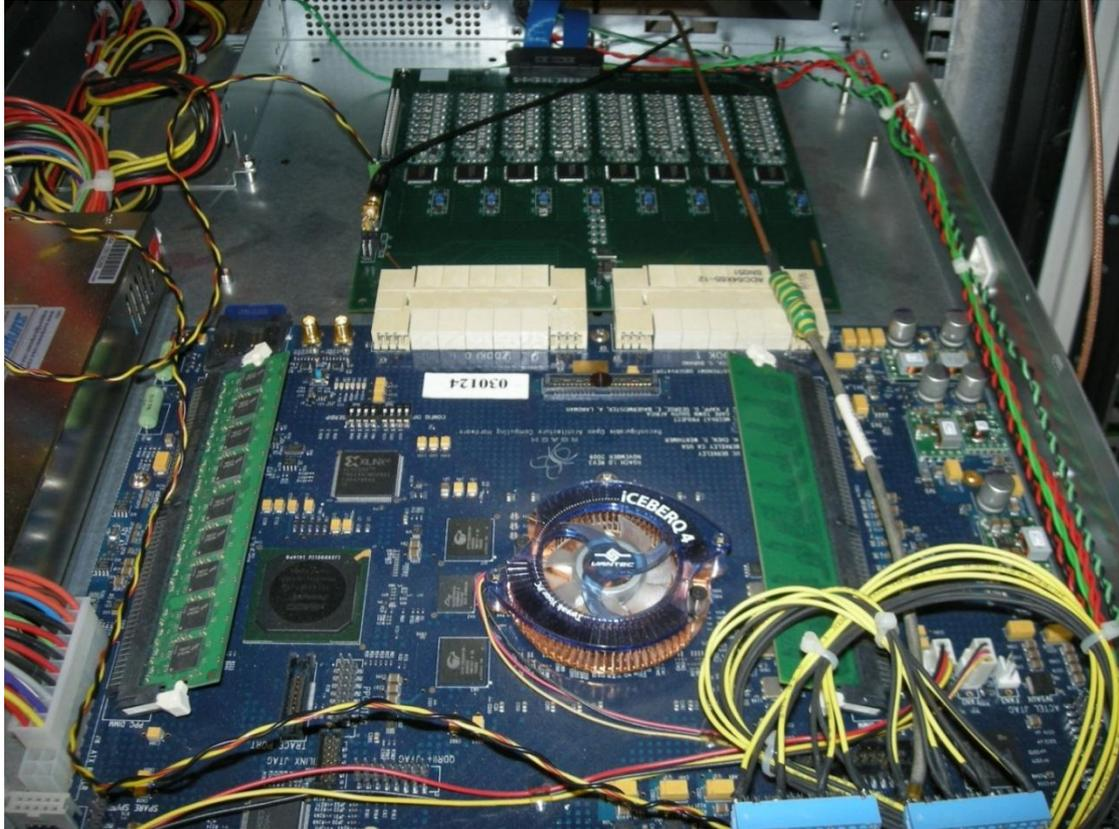
The aim of the Digital Backend is to acquire analog signals coming from the Vivaldi antenna array on the field and to produce in output the result of the Beamformer and the FX-Correlator computed aboard. Two independent parts of the firmware will produce output of 32 bit and 64 bit to allow the study of some quantization effect over the digital chains. The firmware has been designed starting by an already tested part which is a F-engine working as follow:
