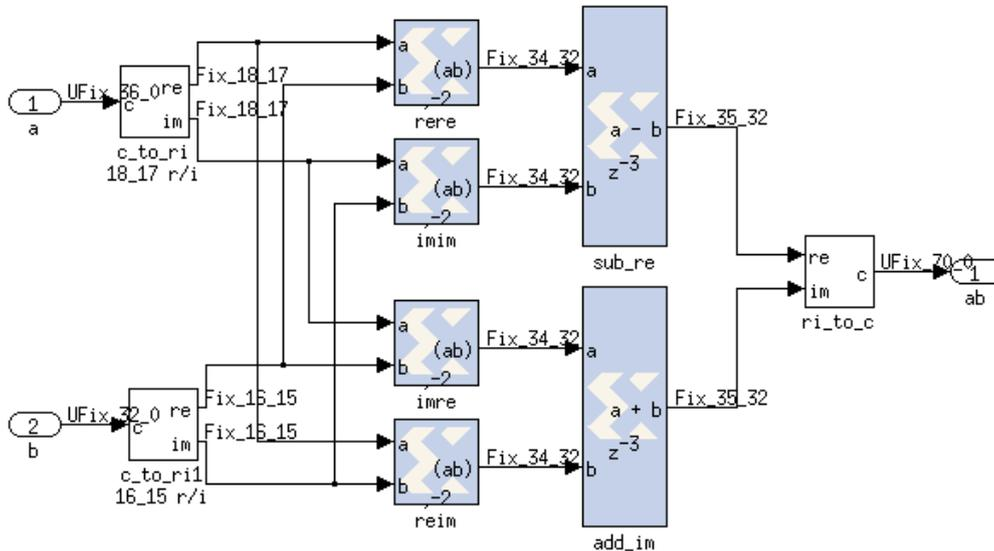
Each stage of multiplier is grouped in subsystems and shown as in the follow picture in the top level Simulink model file.
