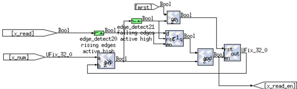
A high level control logic must exist to implement the machine state that serializes the output data. The next picture shows the logic that allow the FIFO-H read enable to start at first, then the FIFO-H, and last the FIFO-X. At the end it is needed to present to the data bus of the packetizer also the output of the beam-former accumulators.
