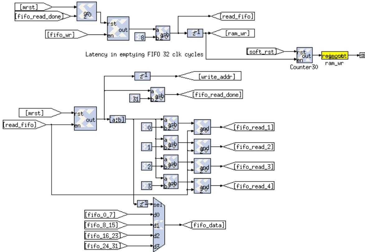
The next picture shows the result using the simulation logic blocks instantiating a constant number for each spectra in the right order. Considering the latency clock cycles when reading data from a FIFO, the 32 frequency channels stored in the DRAM is a ramp between values 0 and 31.
