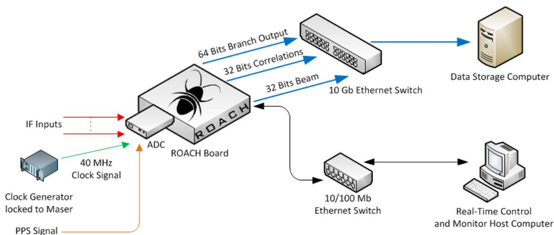
The overall backend architecture is represented above. The IF analog signals arriving from the MAD optical receivers are sampled by the ROACH's ADC, then an onboard processing logic computes the FFT and makes auto correlations and cross correlation products of the interested frequency channel and the beam formed. These data arrives to the storage system via high speed 10 Gbit/s links, while the management is driven by a separate Ethernet link.
