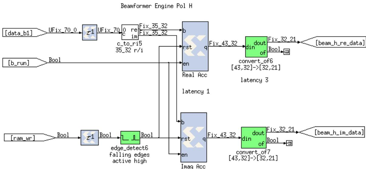
The output of the accumulator which grows up a bit for each sum (worst case) must be quantized due to the limited bandwidth. We have decided to have an output beam formed made by 64 bit for the complex number (32 for the Real part, 32 for the Imaginary part).
