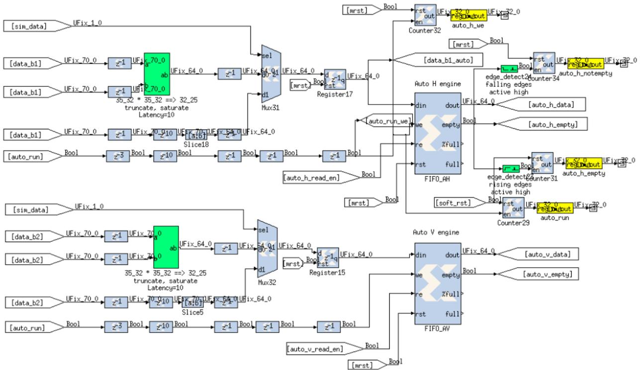
Each single result is stored to a FIFO ready to be sent to the 10 Gbit packetizer. A “FIFO Empty” signal will tell if the FIFO is empty or there are still complex values to read. The X-Engine that computes the cross-correlation products (interference fringes) is equal to the previous engine unless the product factors are not the same values but the frequencies of different antenna of the array. In any case, the output of the green block is internally quantized to match the 64 bit constraints.
