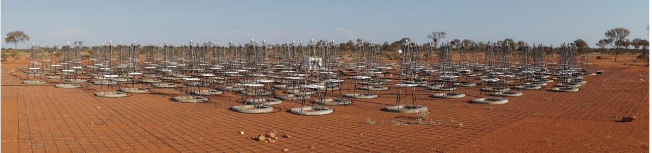
The AAVS1 Main Station, 256 SKALA2 antennas
